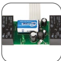
Two built-in relays for currents up to 8 A
