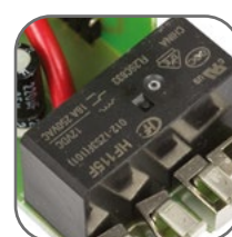
Built-in 16 A relay
