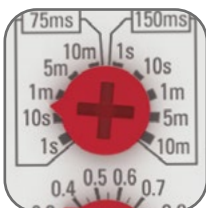
Adjustment interval presets delay time for the mode shutdown «star»
