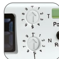
Setting of the number and time of the reclosings
