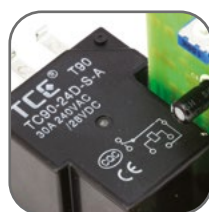
Built-in 25 A relay
