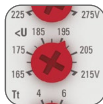
Possible adjustment of the undervoltage value
