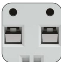
The electrical protection shutter of the terminal
